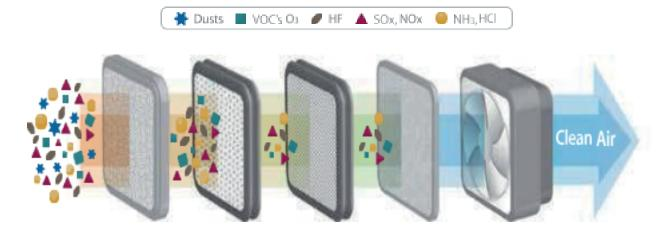
Pre-Filter SAFER -1 SAFER -2 SAFER -3 Blower
